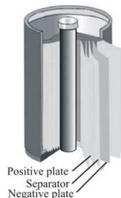
A rechargeable nickel-cadmium cell in a jelly roll arrangement and separated by a layer soaked in moist sodium or potassium hydroxide
